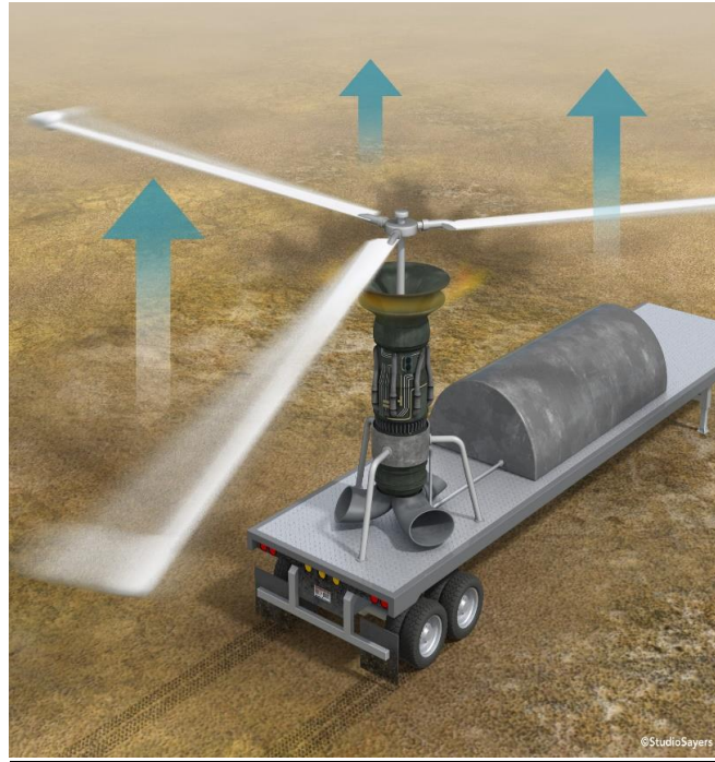
Figure 8: Conceptual conversion of turbojet into turboprop (or turboshaft) system
