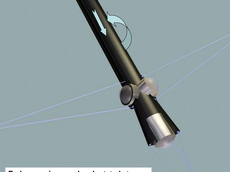
Endoscope is moved and rotated at known rates for 3-D "image from motion"
